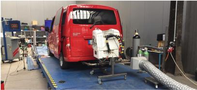
**Fig. 4.** Nissan NV200 Evalia on a dynamometer
